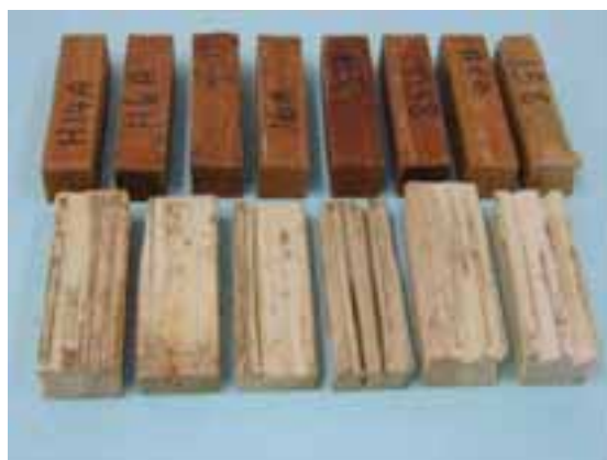
Plate 19b. K. senegalensis and pine feeder block. Note block 158 with slight damage
