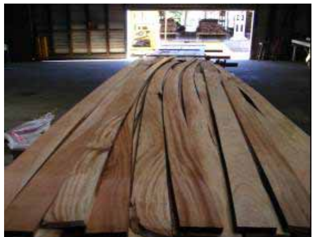
Boards with excessive spring
