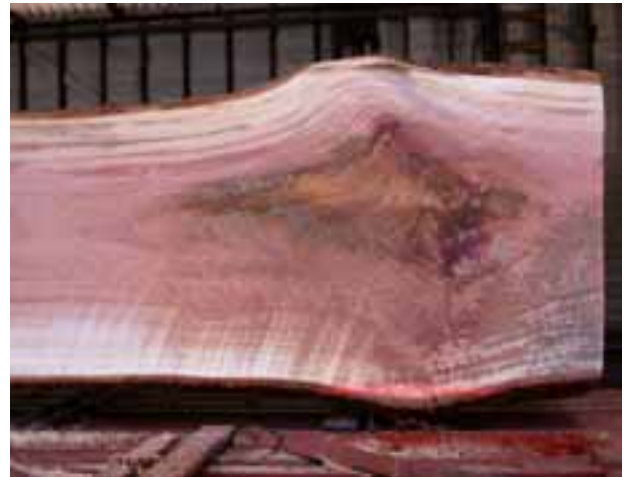
Plate 16. Decay in the inner heart which has entered via a rotten branch stub
